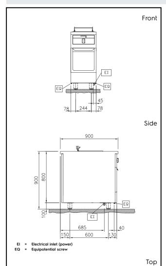
Electric Supply voltage: 400 V/3N ph/50/60 Hz Total Watts: 10 kW **Key Information:** Number of wells: Usable well dimensions (width): 240 mm Usable well dimensions 225 mm (height): Usable well dimensions 380 mm (depth): Well capacity: 12 lt MIN; 14 lt MAX Thermostat Range: 100 °C MIN; 180 °C MAX External dimensions, Width: 400 mm External dimensions, Depth: 900 mm External dimensions, Height: 800 mm Net weight: 75 kg On Base;One-Side Configuration: Operated
